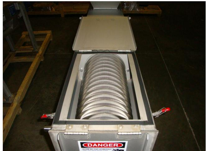
washed out by the stainless steel spray-bar assembly. The washed solids are then conveyed to the discharge end fitted with a “weighted” gate, where the solids are compacted prior to being discharged to a dumpster and then transported to a landfill.
